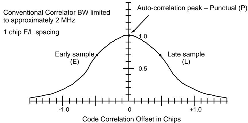
As the E and L correlator samples are spaced 1 chip apart, this places them on the steepest part of the autocorrelation E and L slopes. This placement provides greater sensitivity to changes in the correlation delay-lock-loop (DLL). The E and L samples are differenced to create the appropriate DLL loop feedback for maintaining code lock. Thus, when the E-L difference is zero, the P correlation will be at its peak.
