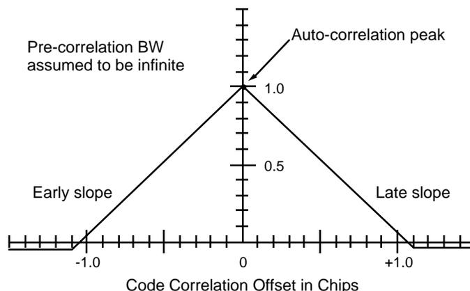
The auto-correlation peak is maintained by continually adjusting the locally generated code for peak correlator output. The unlimited BW provides a sharp correlation peak and steep early/late slope which facilitates accurate error correction for the code-lock-loop (also called Delay Lock Loop).
