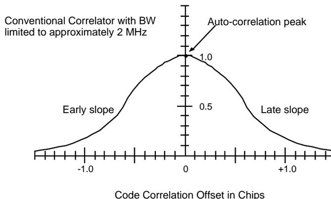
There are various problems associated with single correlator sampling, especially for a 2 MHz BW limited receiver as illustrated in Figure 7 above. As can be seen, the BW limited correlation function is almost flat at the peak. This creates “wandering” at the peak resulting in significant ambiguity in determining the actual correlation peak as well as sensing the early/late slope for error correction. This correlation ambiguity directly translates into range measurement ambiguity.
