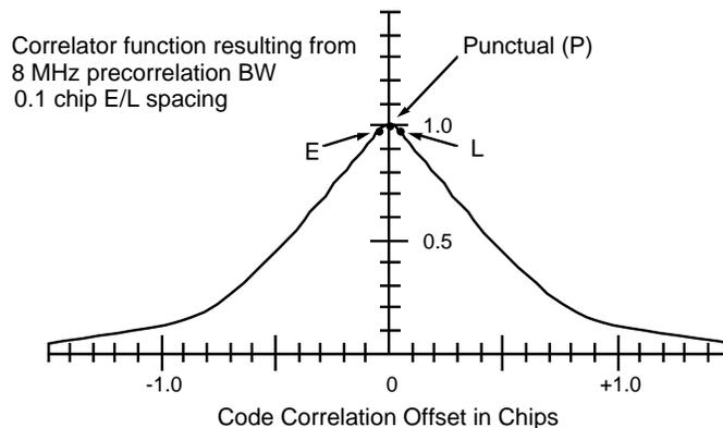
NovAtel’s Narrow Correlator tracking technology is “dynamically adjustable”. This means that the correlator spacing is initially wide for fast acquisition and reacquisition purposes (1 chip spacing), followed by a narrowing down to 0.1 chip spacing for higher accuracy tracking and multipath rejection.
