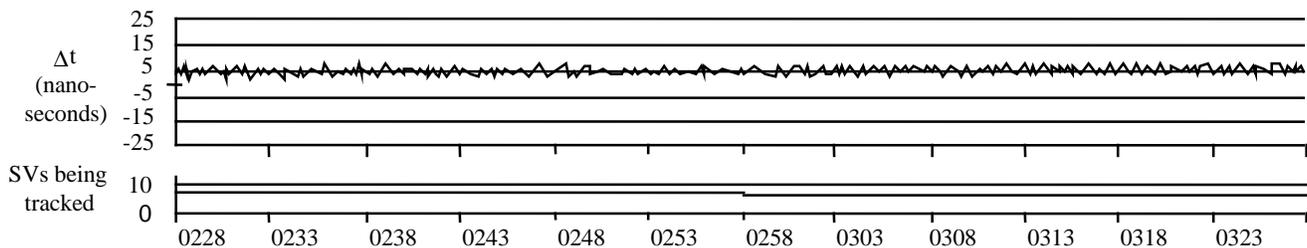
The 1-PPS timing stability is directly related to the reference oscillator stability. The timing improvements realized by the NovAtel OCXO option will ensure more precise data sampling times which in turn provide more accuracy and confidence in pseudo-range and doppler measurements.
