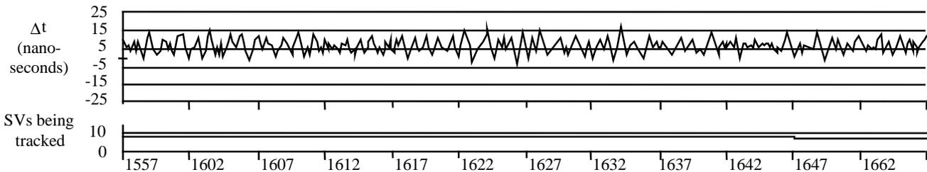
The second set of test data compares two GPSCards, each using the NovAtel OCXO option. This set of measurements shows a significant improvement in timing differences between the two GPSCards. Test results are illustrated in Figure 2 below.
