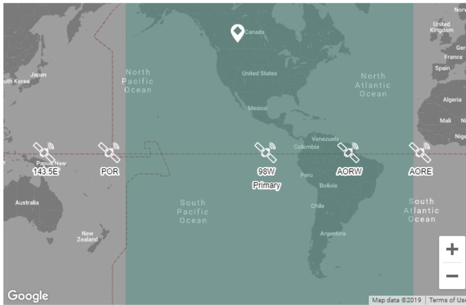
Figure 4: Example Coverage by Primary Geo Satellite / TerraStar Beam for a Specific Location<sup>4</sup>
